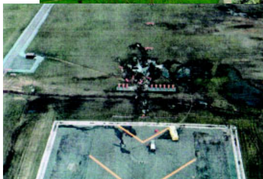
Photos above show two accidents involving airfield obstructions: the F-16 mishap at Misawa and a separate incident where a C-5 wing was broken by a tree near the taxiway at another air force base. Obstructions, including natural and man-made objects, close to a runway pose a greater risk to flight safety. (AFCEA photos)
