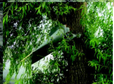
Photos above show two accidents involving airfield obstructions: the F-16 mishap at Misawa and a separate incident where a C-5 wing was broken by a tree near the taxiway at another air force base. Obstructions, including natural and man-made objects, close to a runway pose a greater risk to flight safety. (AFCEA photos)
