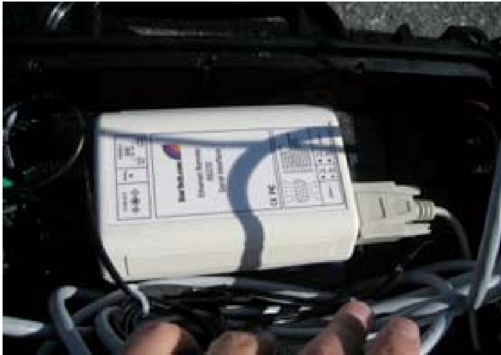
Figure 40. Serial Interface Lens Controller
