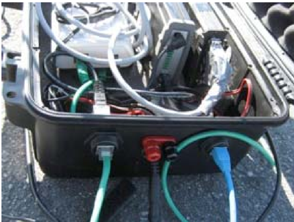
Figure 41. Environmental Housing Configured For ALAN Camera
