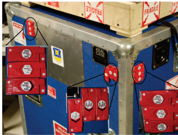
Figure A.3: Shock damage detectors tripped during RIGEX return shipment to AFIT
