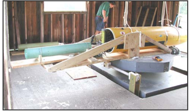
Figure 13. P-2000 configured in front of BPAUV for experiments simulating UUV operations.
