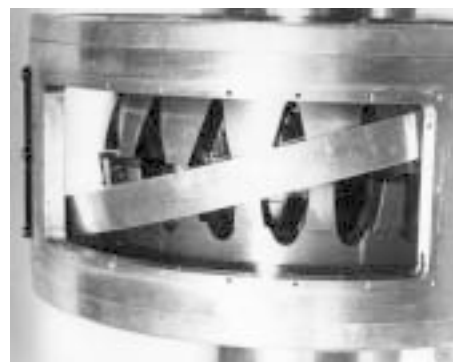
PVT rotor and stator with pericyclic member.
