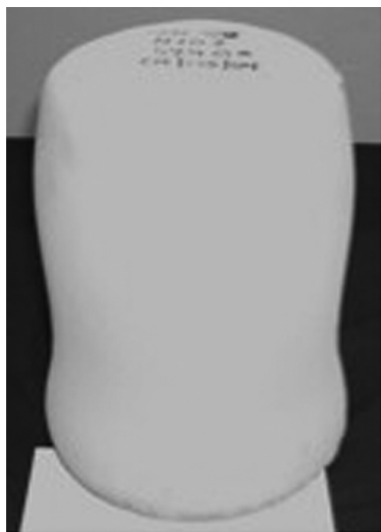
Figure 3. N707 billet in the as sprayed condition before machining.
