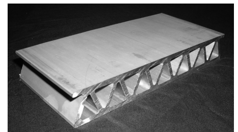
Figure 7. Al-6061 extrusion for light weight blast resistant structure.
