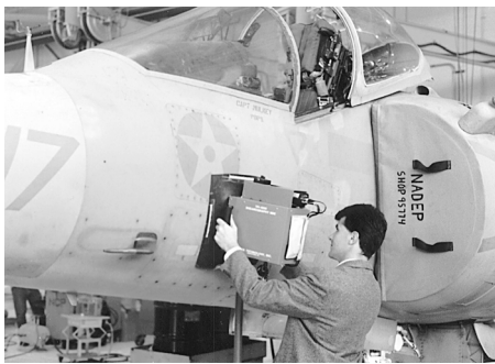
Dr. Bard demonstrates portable field application capability of shearography head on AV-8 Harrier jump jet.
