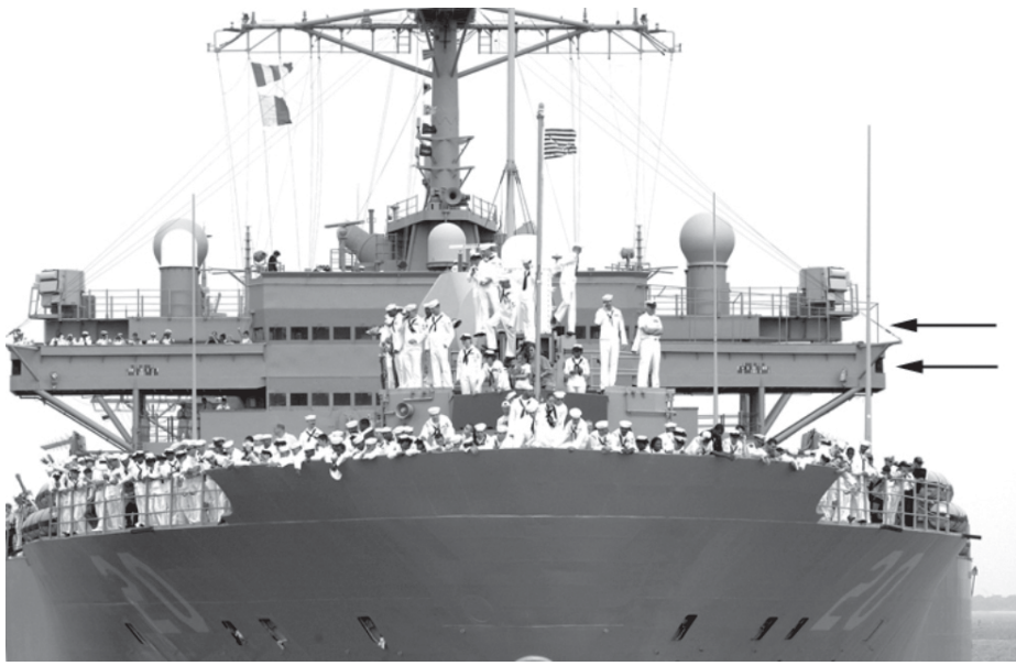
Figure 5. Antenna Platforms on the U.S.S Mt. Whitney (arrowed).
