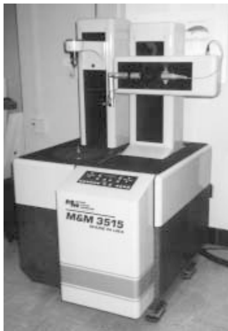
M&M Precision System's new M&M 3515 measuring machine, which is currently housed in iMAST's Drivetrain Technology Center's metrology laboratory. The machine is capable of precise profile, lead, and tooth-spacing measurements on high-performance gears.
