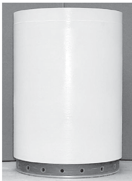
Figure 7. Completed full-scale warhead shroud with attached fragmentation package (after final painting).
