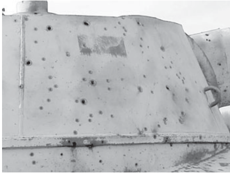
Figure 9. Results from Full Arena Test demonstrating high volume of fragment impact on armored target.
