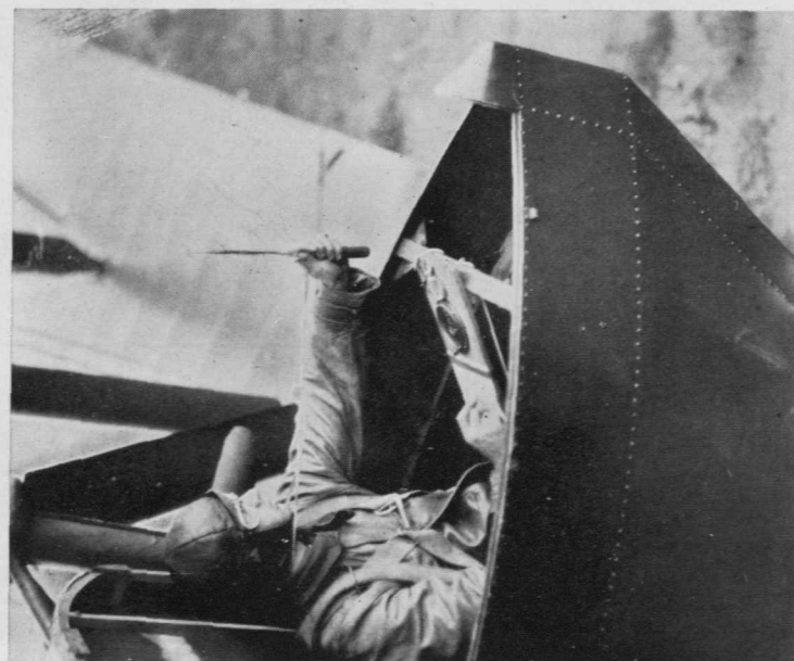
FIG. 6. POSITION OF OBSERVER IN NACELLE AS SEEN FROM THE RADIO COCKPIT. NOTE THE BOARD FOR ALTIMETER, WATCH, AND RECORDS
