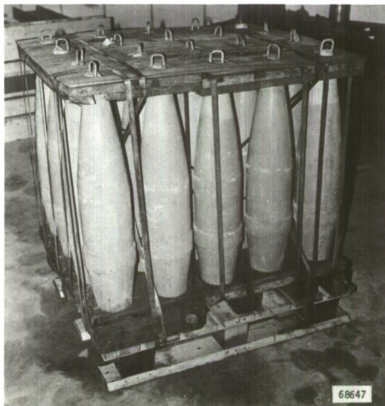
Fig 10 Condition of unit head after all tests. Note nails holding feather edge in position
