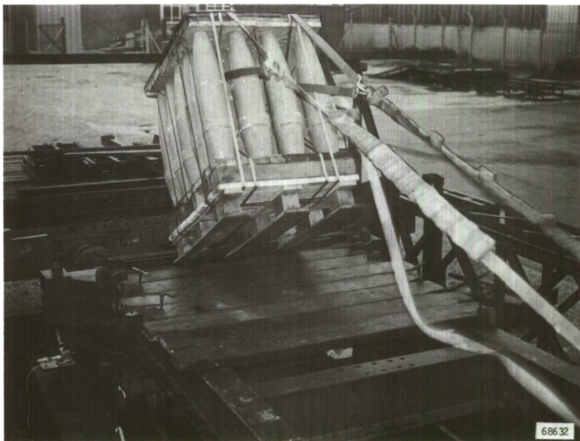
Fig 5 Loose shunting test on MVEE rig. Note electrical timing device velocity at instant of impact, 14.0 feet/second
