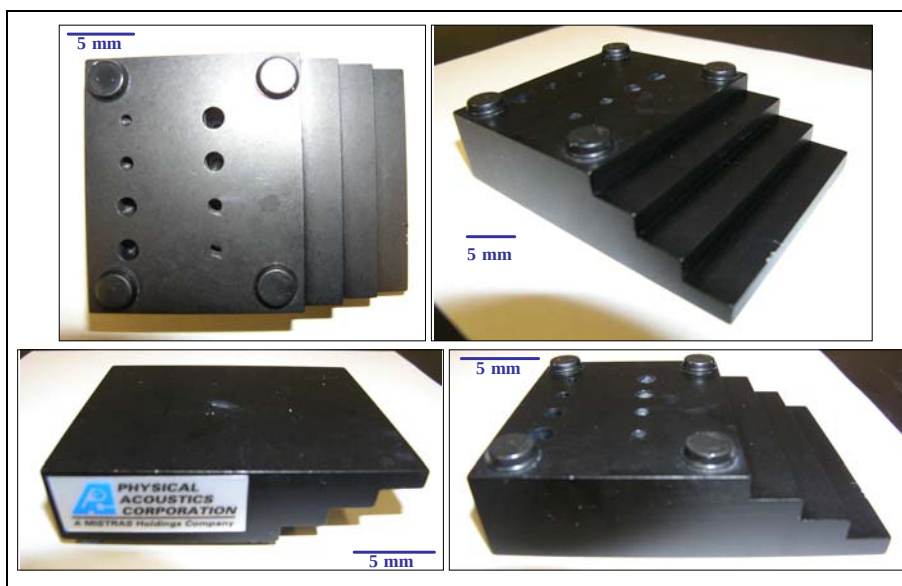
Figure 5. Aluminum standard sample featuring steps and drilled holes.
