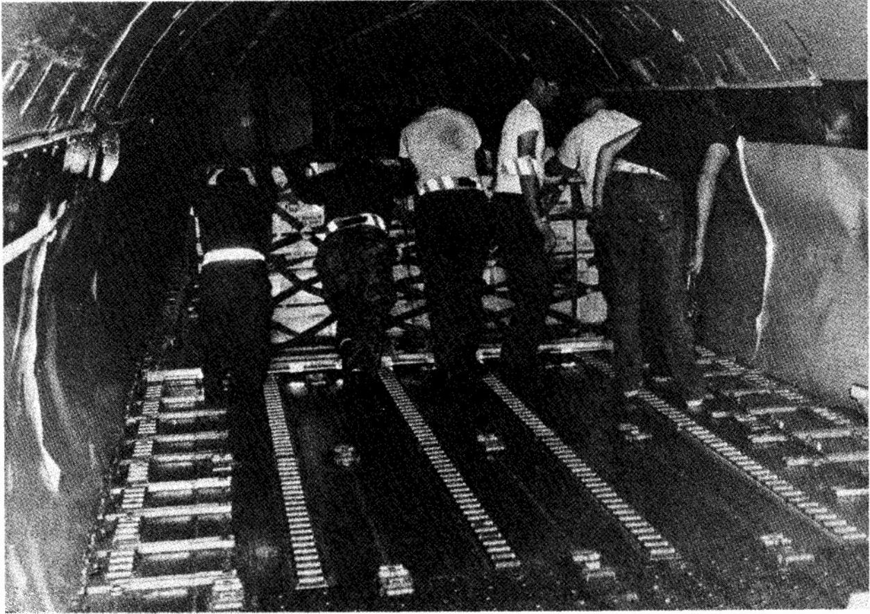
Pallet of 105mm cannon shells being pushed into position aboard aircraft. This aircraft carried 88,050 pounds of cargo on 15 pallets and was loaded in 51 minutes.
