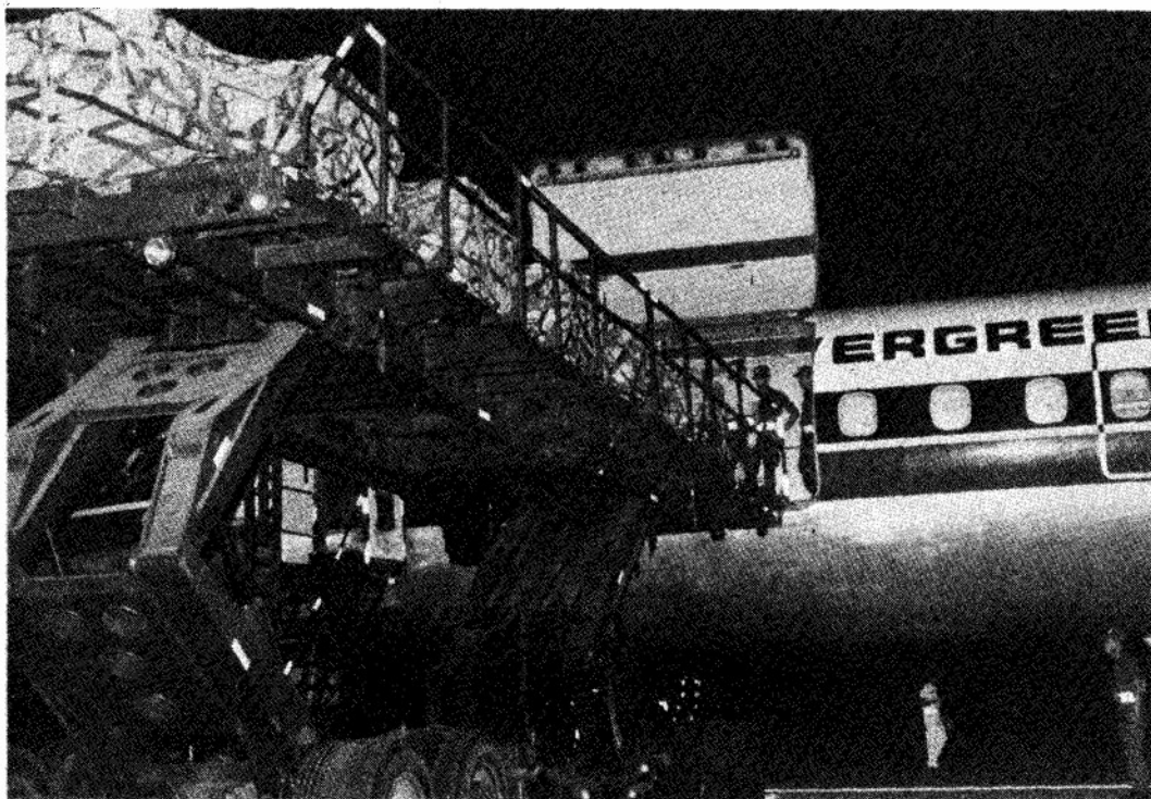
40K Loader with 5 pallets of 105mm cannon shells, positioned to onload Evergreen Airlines DC-8. Each pallet weighs 5,870 pounds.
