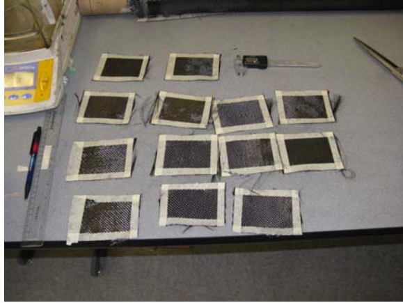
(a) Preforms of heat-treated T300 fabrics with applied processing adhesives
