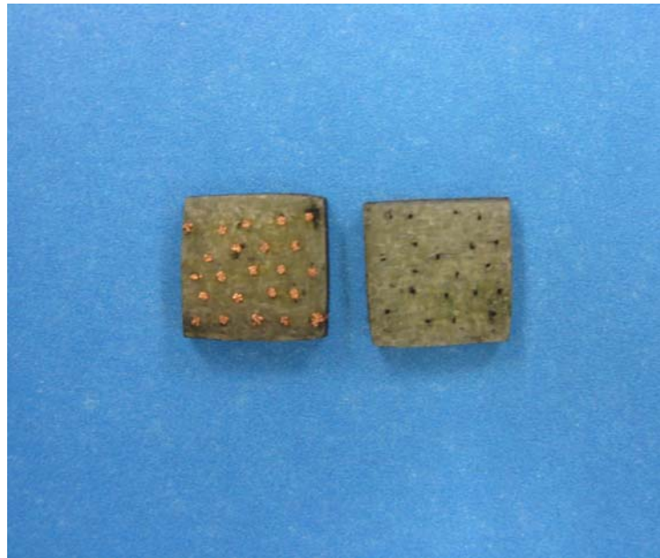
Figure 17. Cured glass fiber/epoxy composite samples with stitched copper wire (0.003 inch diameter) and nanotube yarns ready for thermal conductivity measurement
