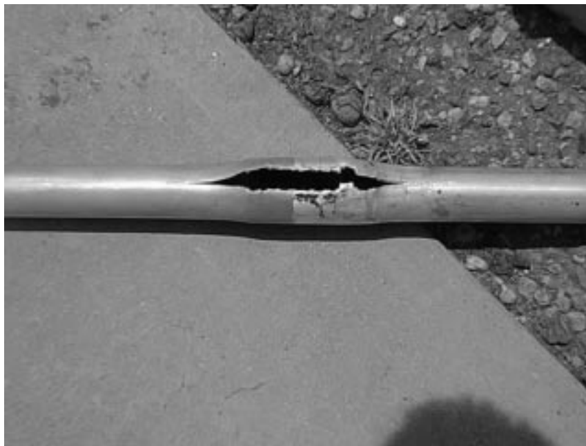
Figure 4.3. Unpredicted longitudinal tearing of the tube.
