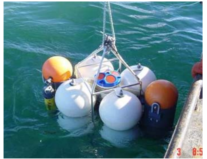
Figure 5: The ADCP in mooring frame with white flotation spheres during deployment. Below the frame is chain and a 226 kg (500 lb) anchor; two acoustic release packages can be seen on the sides of the system.
