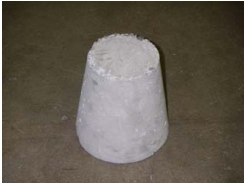
Fig.9 Concrete Tapped Cylinder (15.5(D)x10(D)x5.8(H)cm)
