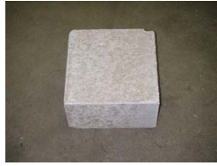
Fig.2 Concrete Cube (17.8x17.8x10.2(H)cm)
