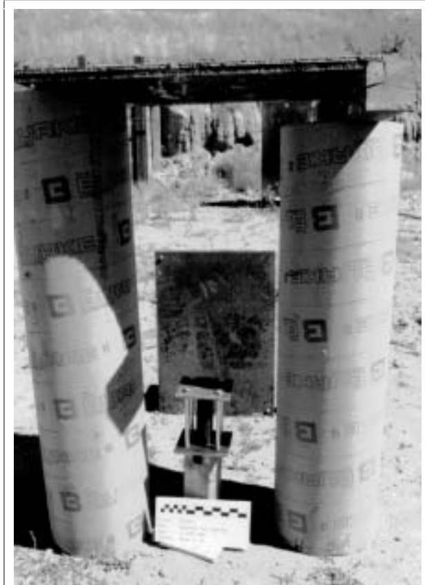
Figure 6. Cook-off fragmentation test.
