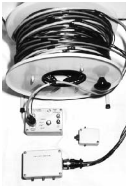
Figure 3. Remote modules attached to 100 feet of cable.
