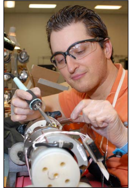
Matthew Butash, electronics worker (student trainee) at Tobyhanna Army Depot, repairs an AIM-9(M) Sidewinder missile guidance and control section in the pre-final area of the shop.
