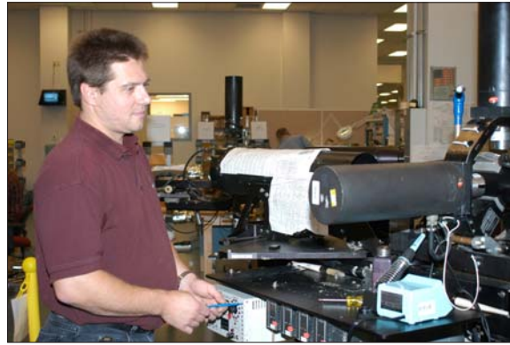
Joseph Marshalek, an electronic measurement equipment mechanic in the Communications Security and Tactical Missile Systems Directorate, uses a radiometer to calibrate the infrared heat source on the Navy Rate Table. The table is used to test the guidance and control section of the Sidewinder missile.
