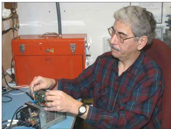
Roy Dudeck, an electronics mechanic in Tobyhanna Army Depot's Avionics-Intelligence Electronics Warfare Systems Directorate, prepares to test an AN/ARC-186 Aircraft Set circuit card. The U.S. Air Force increased the workload for these radios after technicians successfully demonstrated they could overhaul them.
