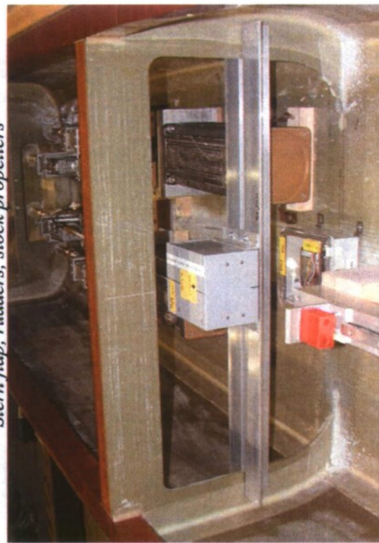
LCG Motions Sensors (2-axis Pitch & Roll, 3-axis Acceleration)
