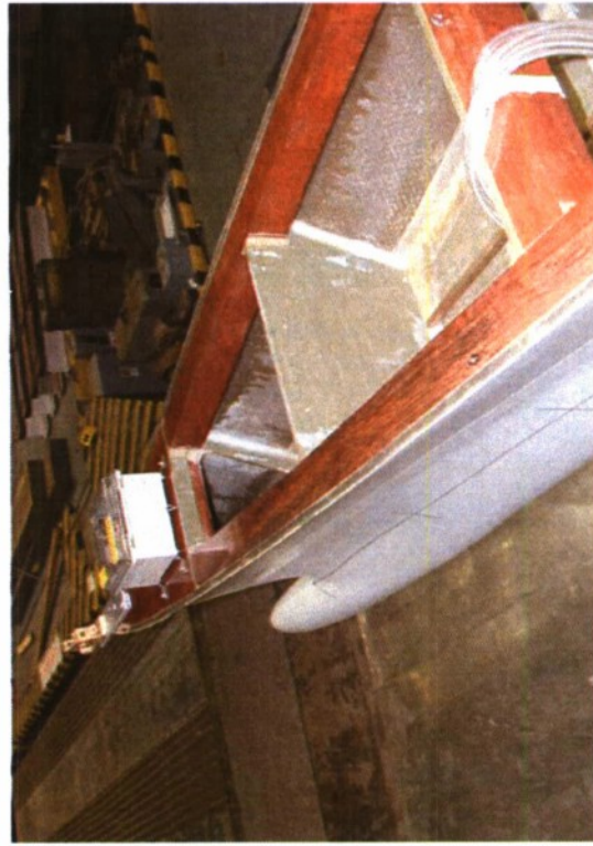
Forward Motions Sensors (3-axis Acceleration)
