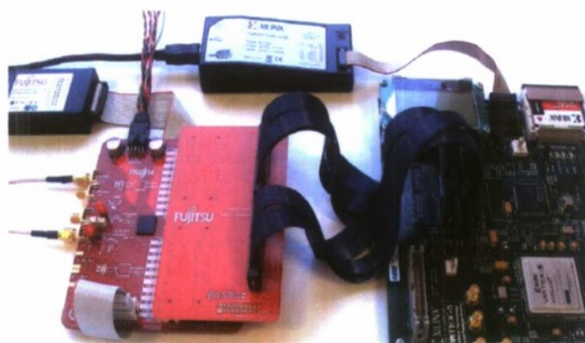
Figure 2.6: Interfacing DAC evaluation board and FPGA evaluation board.
