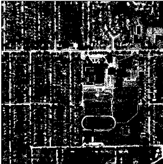
Figure 4.26: When compared to the original satellite image (upper left), the false color composite of the hyperspectral scene (upper right), and the “ground truth” roadway surface object map (lower left), there are six notable road network discrepancies (lower right). 1. These are parking areas identified as road network. 2. The road curves are not handled well. 3. There are two cul-de-sacs that are completely occluded by tree foliage. 4. This roadway does not exist in the “ground truth”. 5. It is undetermined if this roadway exists or not. It exists in the satellite image (upper left), does not exist in the false color image (upper right), and may exist in the ground truth roadway object map (lower left). 6. Road segment is missing.
