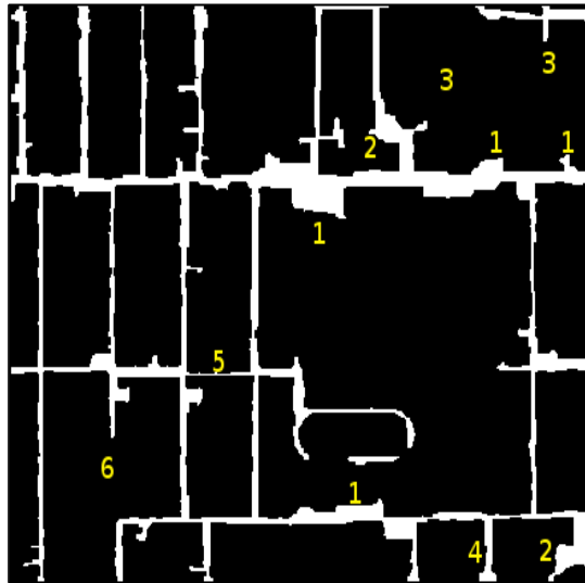
Figure 4.26: When compared to the original satellite image (upper left), the false color composite of the hyperspectral scene (upper right), and the “ground truth” roadway surface object map (lower left), there are six notable road network discrepancies (lower right). 1. These are parking areas identified as road network. 2. The road curves are not handled well. 3. There are two cul-de-sacs that are completely occluded by tree foliage. 4. This roadway does not exist in the “ground truth”. 5. It is undetermined if this roadway exists or not. It exists in the satellite image (upper left), does not exist in the false color image (upper right), and may exist in the ground truth roadway object map (lower left). 6. Road segment is missing.
