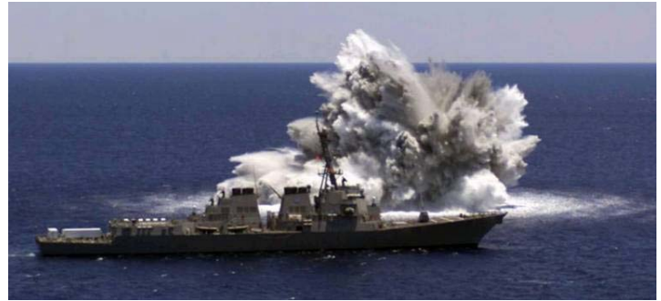
Fig. 13. USS Winston Churchill (DDG-81) Shock Trial
