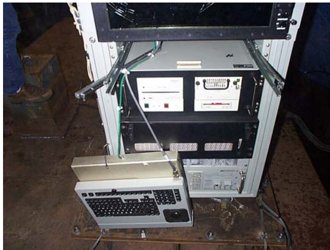
Fig. 10. Keyboard hanging from the broken slider.
