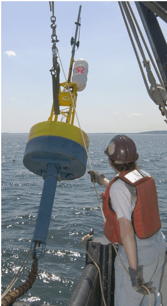
Fig. 5. Deployment of the custom-designed surface buoy at the Scituate site. Buoy is 0.5 m high and 0.9 m in dia. The potted cable is visible at the bottom.
