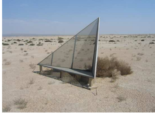
Figure 3.16: An example triangular corner reflector from the NASA Rosamond Calibration Array. [29]
