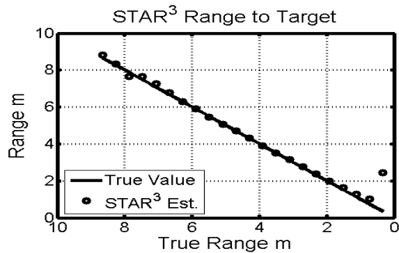
Fig. 4. Simulation of target-ranging measurements from a STAR Cube gradiometer as it homed in on a 14.7 Am 2 magnetic dipole target. All 24 channels had 120 pT p-p random noise.
