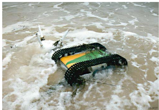
Fig. 2. A Lemming and its sensing whisker
