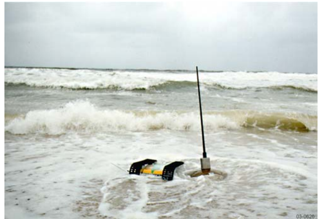
Fig. 1. A Lemming class crawler near a surf zone object.
