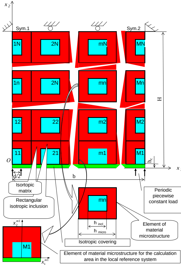
Fig. 2 The transverse deformation of semi-limited matrix with covering reinforced by rectangular fibers. Geometry and scheme of loading
