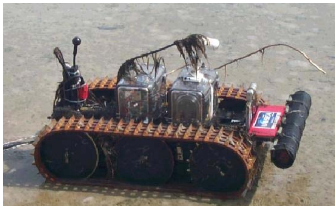
Fig. 1. Robotic crawler with sensor and sampling boxes mounted on top plate. Note the long sampling tube extending beyond the bumper.
