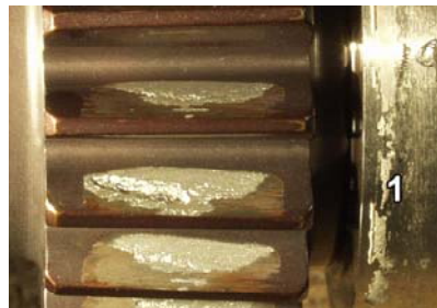
a) Single/few teeth macro-pitting failure.
