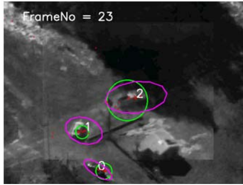
Fig.5. Target detection result at frame 23, by using clustering technique to the objects detected from frame 14 to 23.
