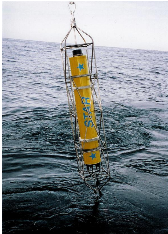
Figure 36. Simple Tomographic Acoustic Receiver electronics package (photo courtesy of Lloyd Green, Scripps Institution of Oceanography).
