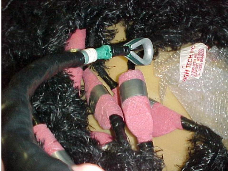
Figure 8. Close up of the VLA hydrophone elements (under pink wrapping), and faired array strength member.
