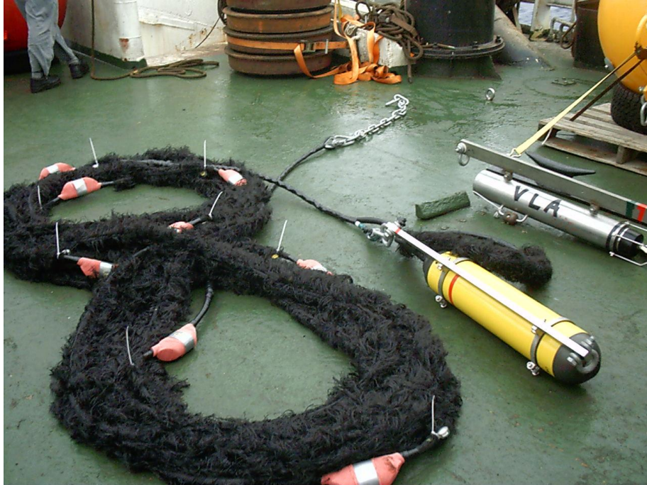
Figure 9. VLA on deck, ready for deployment. The VLA "STARmini" electronics package is connected (yellow pressure housing connected to strength member), and the mooring motion interrogator is also shown (far right). (Photo courtesy of Linus Chiu, NTU).
