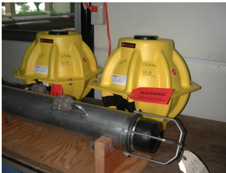
Figure 12. Mooring motion components: the WHOI Acoustic Interrogator (foreground), and two Benthos transponders (background).
