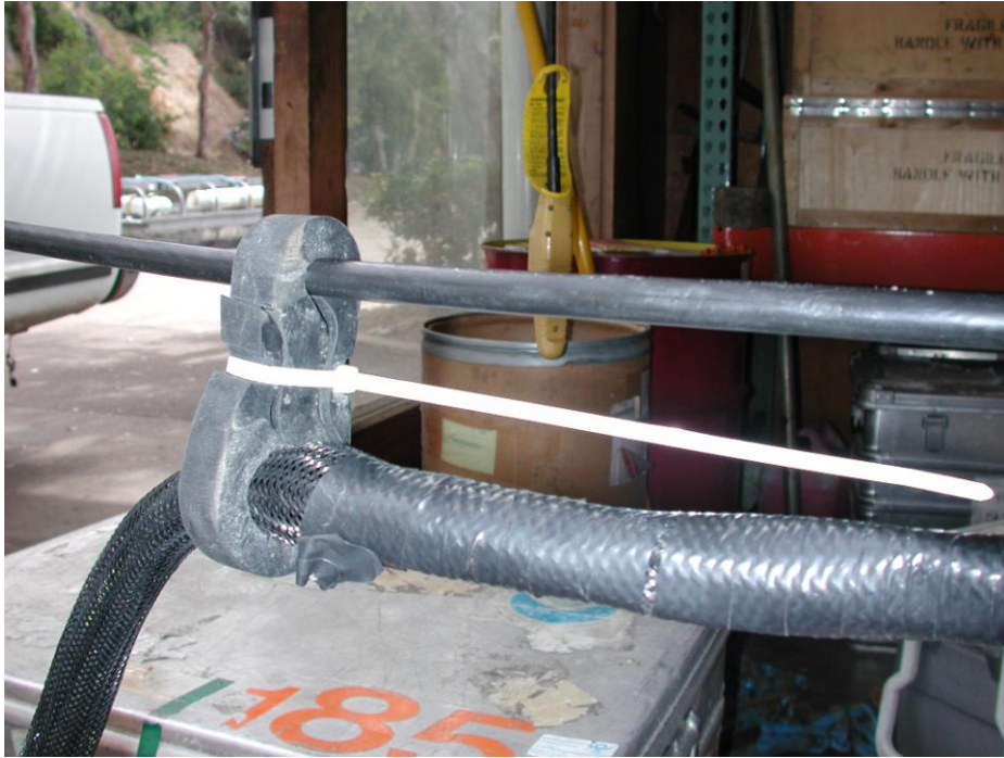
Figure 37. The rubber isolator used to mount the STAR array cable (bottom) to the jacked wire-rope (top) for the 4-element, 32m aperture STAR array.
