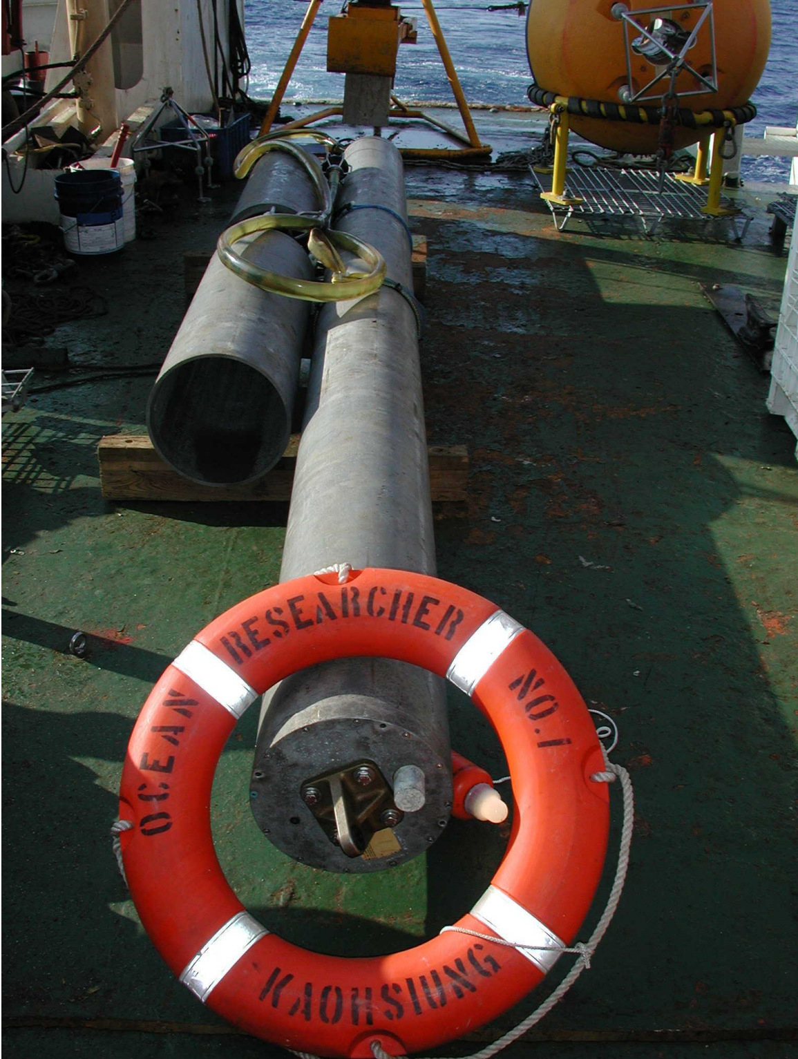
Figure 29. 400 Hz Tomography source ready for deployment at the B1 mooring site.
