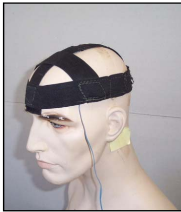
Figure 3. Headband designed to hold C-2 tactors.
