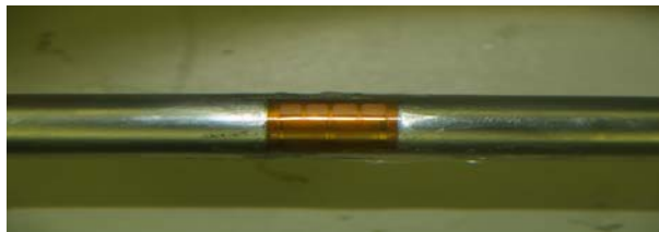
Figure 3: Strain Gauges Attached on a Steel Bar
