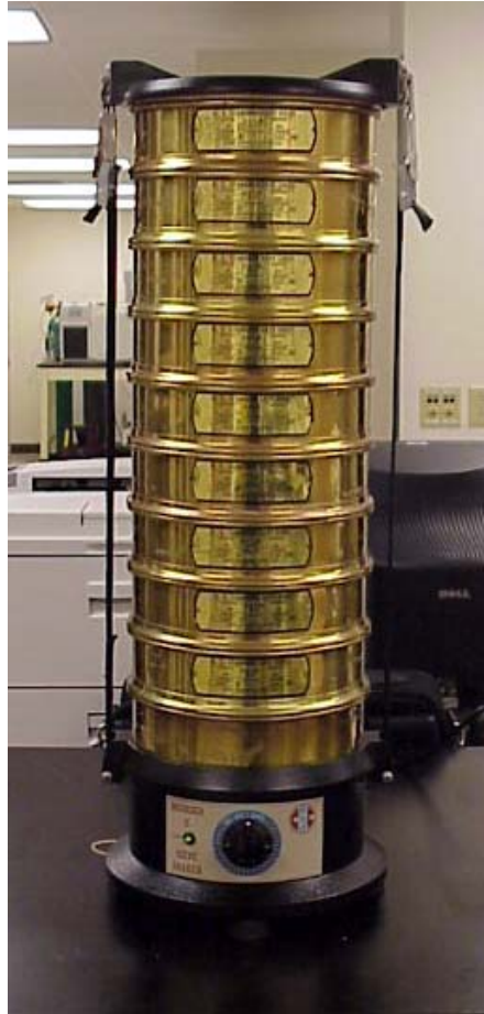
Figure B-2. Sieve Shaker Set-up
