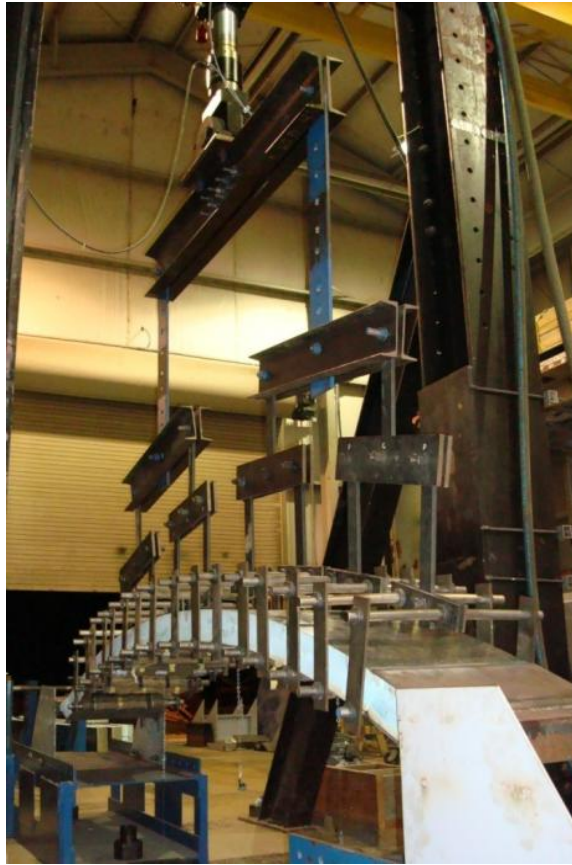
Figure 2. SEFCP being tested in load tree.
