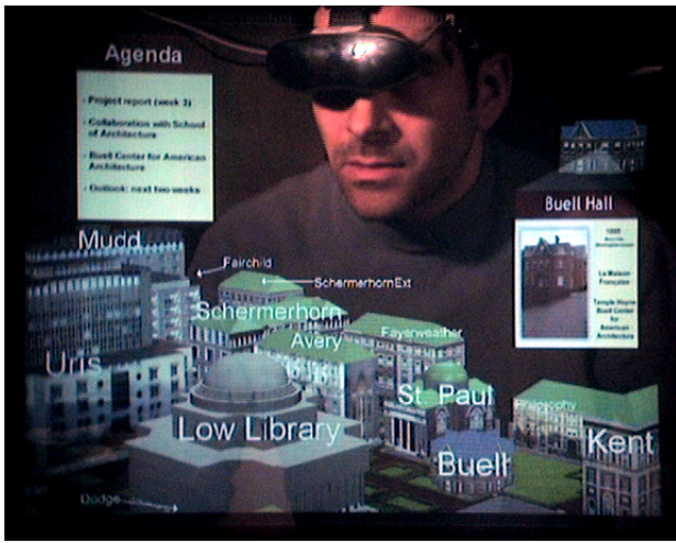
Figure 10: View management in a collaborative system (imaged through see-through head-worn display). Labels are laid out dynamically to annotate the buildings of a campus model as seen by the observer. UI elements avoid overlapping the colleague's head and the campus model.
