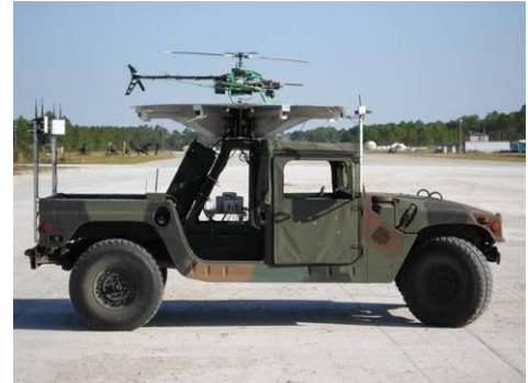
Figure 14. The AUMS platform mounted on a remote-controlled HMMWV and supporting a Mongoose UAV.
