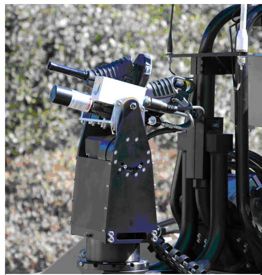
Figure 11. A less-lethal NROWS mounted on an MDARS vehicle.
