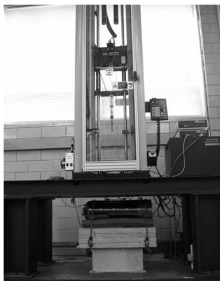
Figure 2 – Instron drop tower used to simulate impulsive loads.
