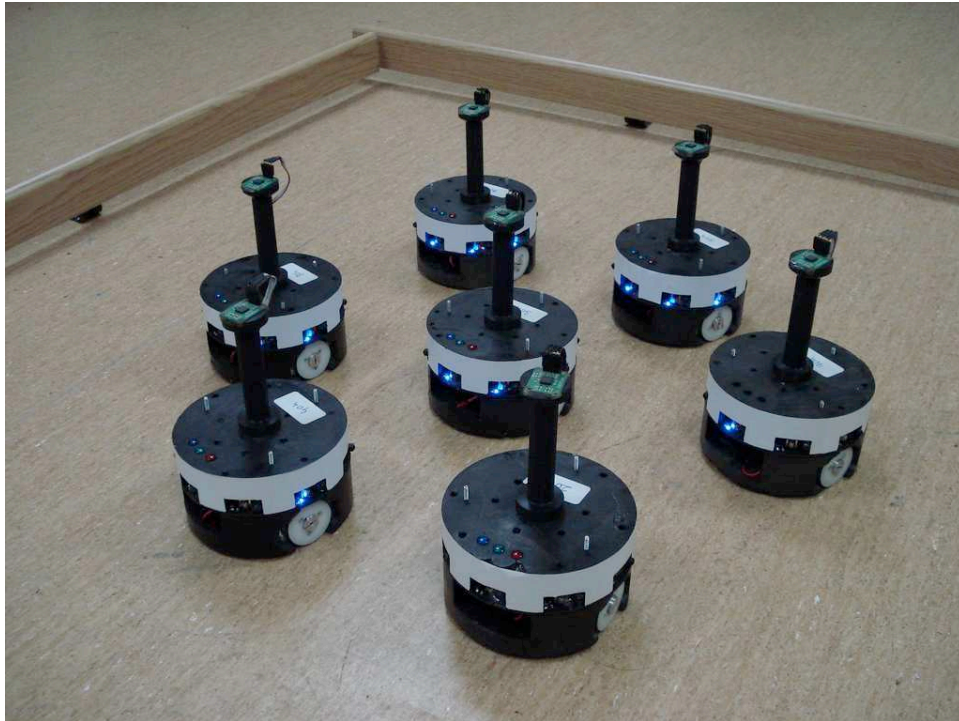
Figure 2.3: Kobot . A group of seven kobots designed by a group from the Middle East Technical University in Ankara, Turkey [3].
