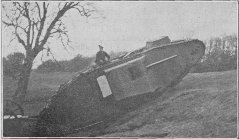
FIG. 1. FIRST BRITISH HEAVY TANK
