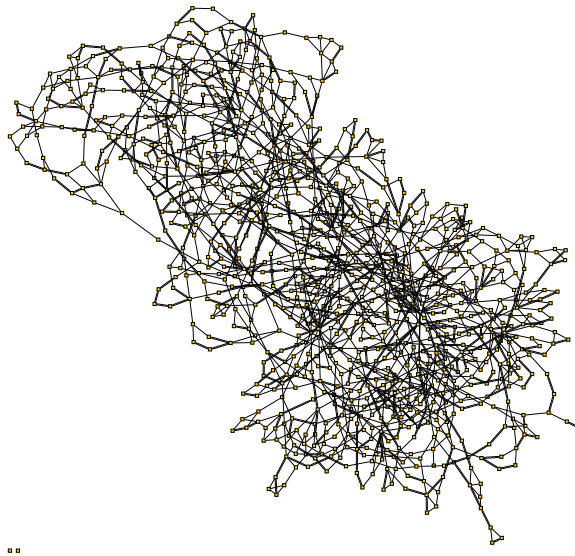
Figure B.19: Obfuscated Circuit Variant Graph after applying 500 iterations, 4 replacement sizes, and TFTTTT library generation option to circuit R17' + C17 + R17'' . (1049 gates, 336 levels)
