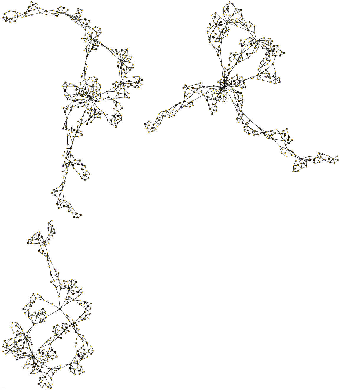
Figure A.5: Obfuscated Circuit Variant Graph after applying 1000 iterations, 3 replacement sizes, and FFFTTT library generation option to circuit C17+C17+C17 . (943 gates, 155 levels)
