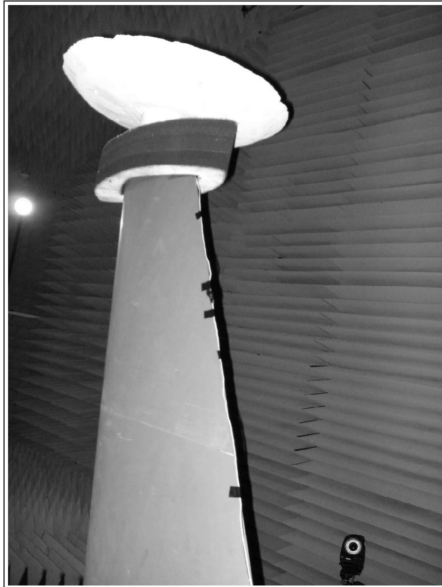
Figure 3.4: AFIT anechoic chamber target mount pedestal. The photo was taken from the backside of the pedestal, where the Styrofoam mount that supported all of the targets can easily be seen. The power cable that drove the motor unit ran through the Styrofoam support and was looped inside of the elliptical foam absorber to suppress its interference effects on the backscatter. The cable can be seen running down the backside of the pylon.
