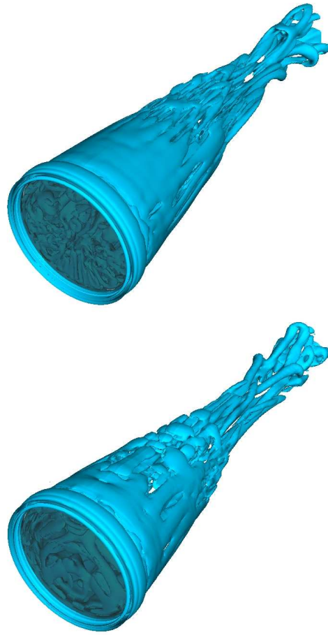
Figure 6.2 Instantaneous iso-contours of Q = 0.05 from FSM calculations using kh = 32 & \beta = 0.002 (top) and kh = 16 & \beta = 0.004 (bottom); perspective view from inflow towards outflow; base of body shaded grey.
