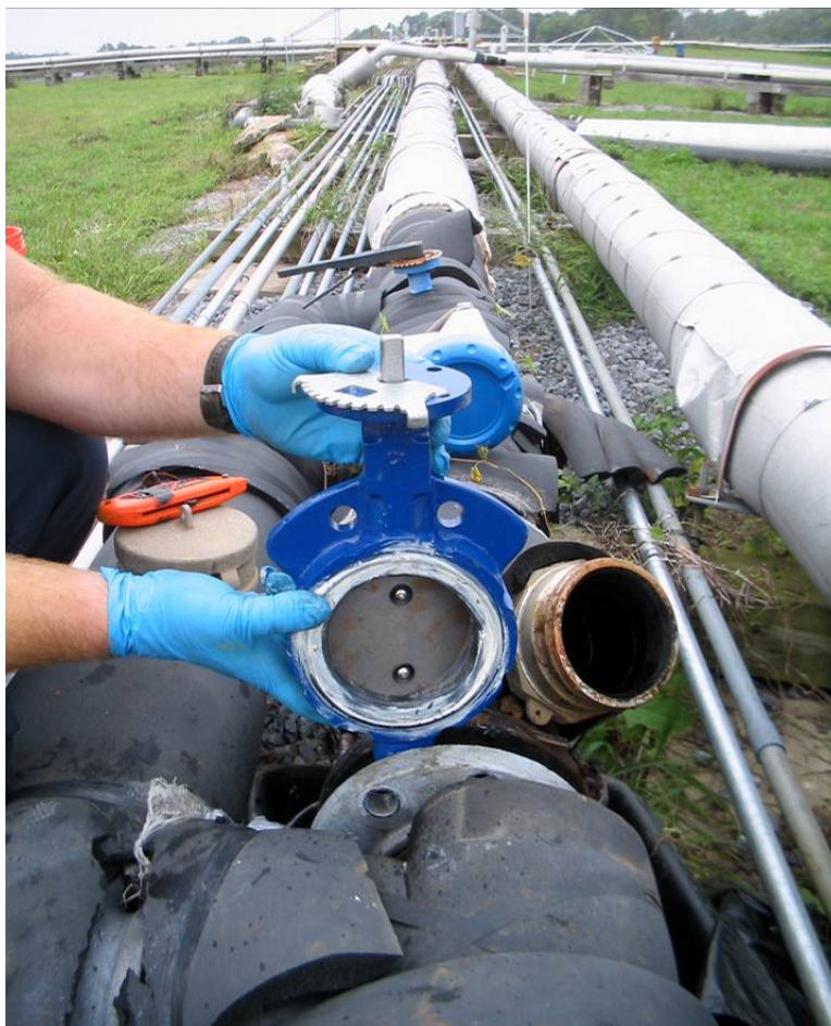
Figure 22. Photograph of test coupon about to be inserted into the west header.
