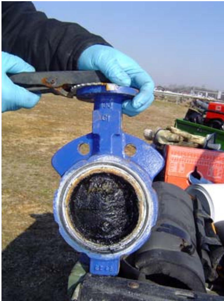
Figure 23. Photograph of the test coupon after 6 months in the west header.
