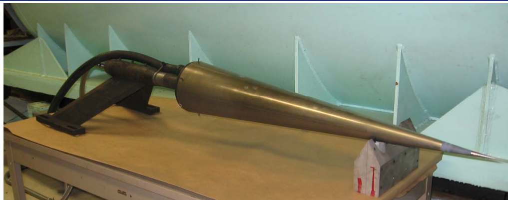
Injector installed in a ~1m long 5-deg cone to be tested in T5
