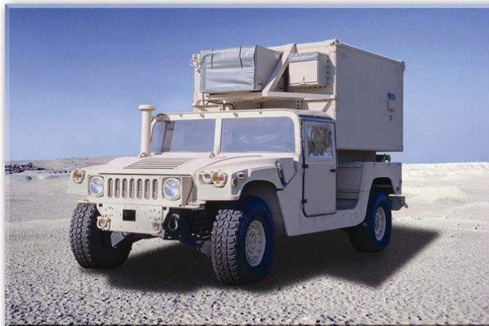
The JNN-N equipment suite is comprised of a shelter mounted on a High Mobility Multi-Wheeled Vehicle, Ku band SATCOM trailers, transit cases and Hub Sets.
